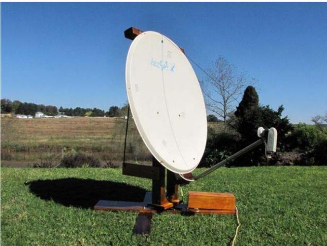
Left - the dish reflects the incoming signal onto the receiver which is at the end of the arm pointing right and is called the LNB.
