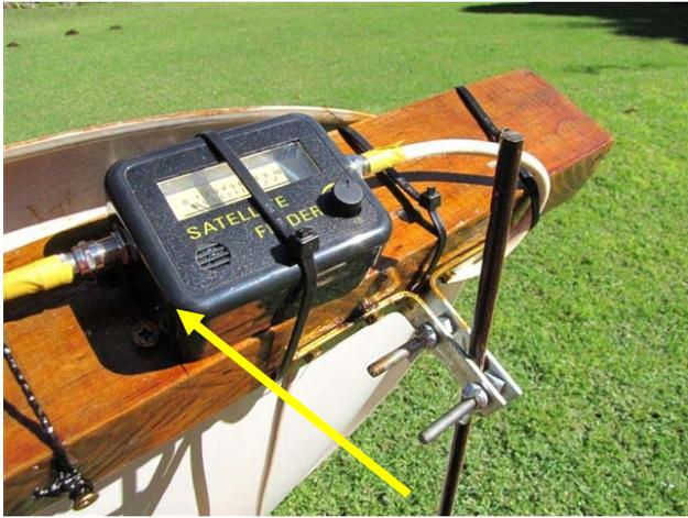
Left - Another view of the signal meter. Note also the altitude fixing bar and clamp
