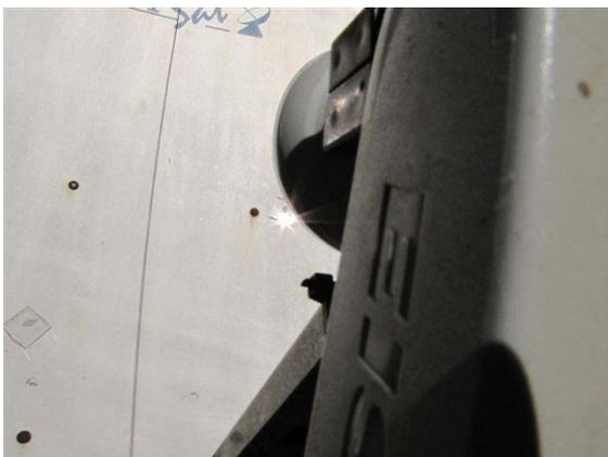
Left - view from LNB back to dish. Note the Perspex squares used to check that the LNB is correctly aligned, and the shadow of the black string.
