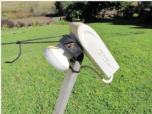
Left - the old LNB receiver from the disused satellite dish still works after many years sitting in the junk box. The black string helps to keep the LNB in place and is also useful when aiming the dish.
